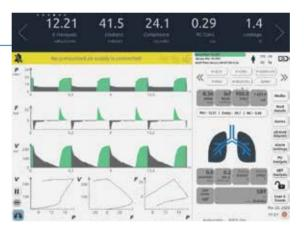
It allows to monitor/ see the dynamic state of lung with lung diagram, which provides intelligent ventilation monitoring.
